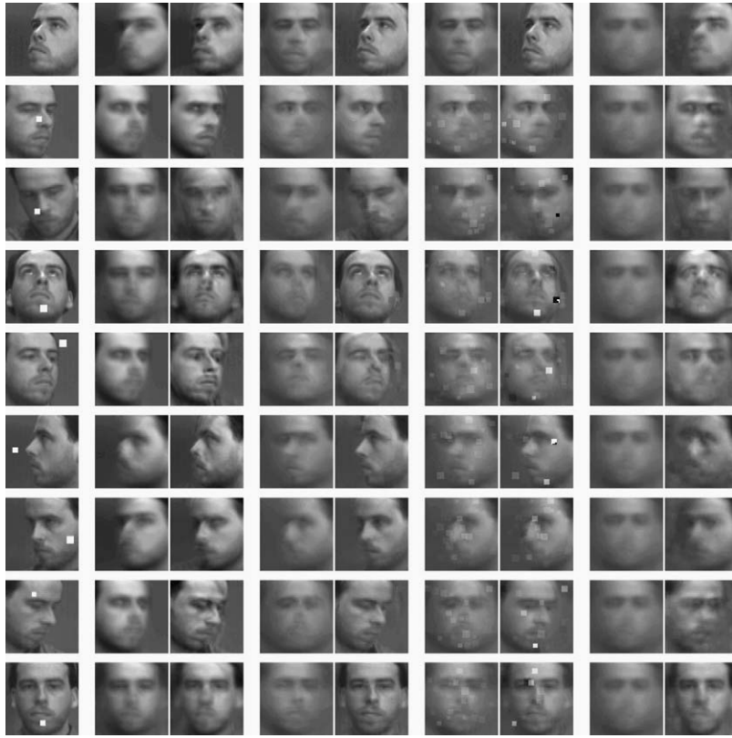
Fig. 5. Sample results of multi-view face modelling. From left to right: original face image, mean vectors and reconstructions of (1) view-based eigenface method, (2) Algorithm 2, (3) Algorithm 1, and (4) batch-mode PCA, respectively. Results are shown for every 20 frames of the test sequence.
